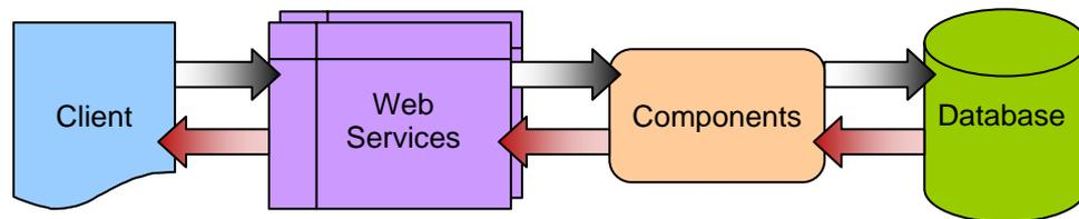
The Self-Service Kiosk passes requests through HTTP or HTTPS to the MyID Data Source and MyID Process Driver web services; both services are required for full operation. The web services communicate using DCOM with the MyID components on the application server; these components provide the business logic and communicate with the MyID database. Responses are returned to the client through the MyID web services.
